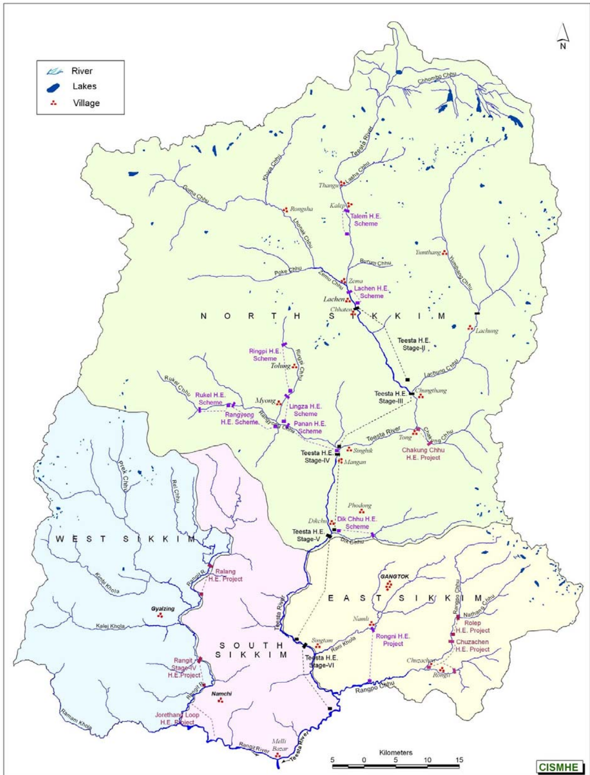
Fig.6 Proposed hydro-power development model in Teesta river basin in Sikkim
