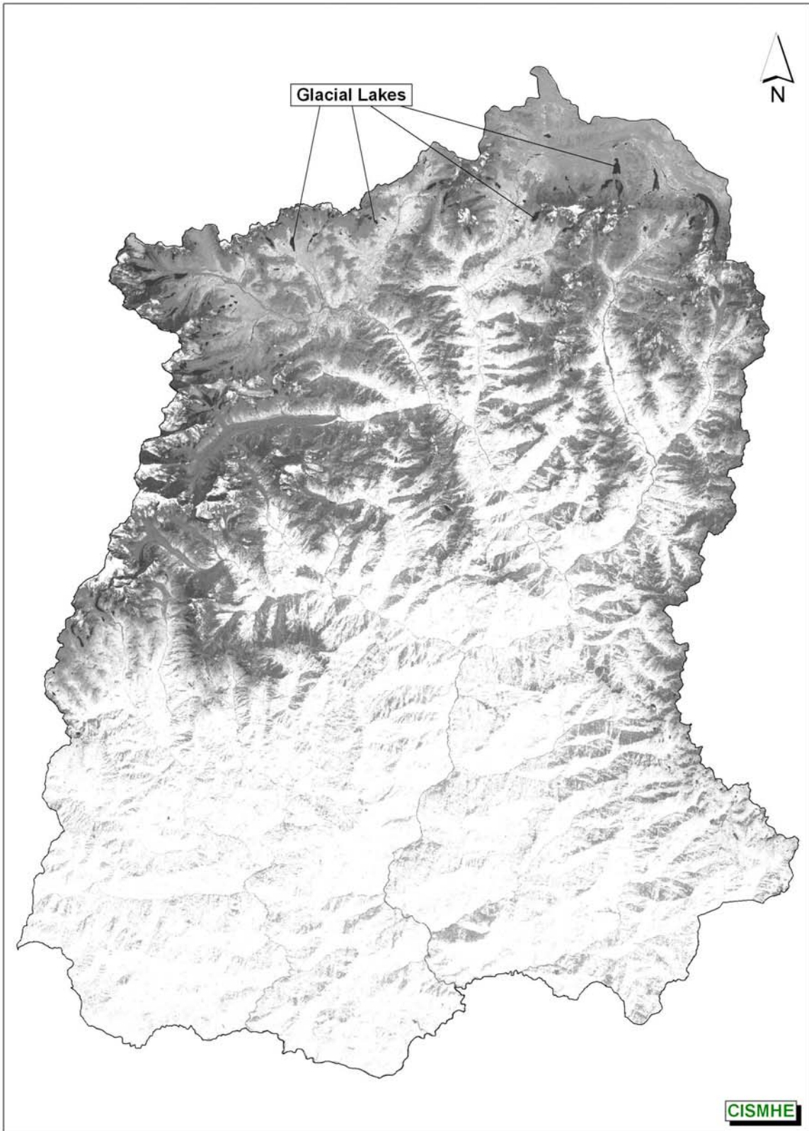
Fig.3.14 Subset and band ratio image of Landsat-7 ETM+ of December, 2000 to show glacial lakes of Teesta basin in Sikkim
