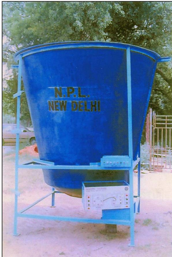
Fig.5 Sodar antenna
